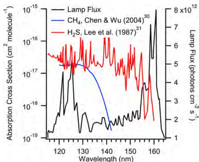
**Figure 2.** Absorption cross sections (cm<sup>2</sup> molecule<sup>-1</sup>, left axis) for CH<sub>4</sub> (blue)<sup>30</sup> and H<sub>2</sub>S (red)<sup>31</sup> and lamp flux (cm<sup>-2</sup> s<sup>-1</sup>, right axis) (black, provided by the manufacturer) as a function of wavelength in the range of the lamp's peak emission.
