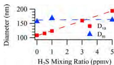
**Figure 6.** Volume-weighted mode mobility diameter ( $D_m$ , nm) (blue) and vacuum aerodynamic diameter ( $D_{va}$ , nm) (red) as a function of initial  $\text{H}_2\text{S}$  mixing ratio.
