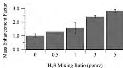
**Figure 4.** Total organic aerosol mass loading enhancements as a function of  $\text{H}_2\text{S}$  mixing ratio. Enhancements are calculated relative to the average 0 ppmv  $\text{H}_2\text{S}$  mass loading. Error bars signify 2 standard errors of the mean centered at the average mass loading. Only one experiment of 0.5 ppmv  $\text{H}_2\text{S}$  was conducted due to subsequent failure of the deuterium lamp.
